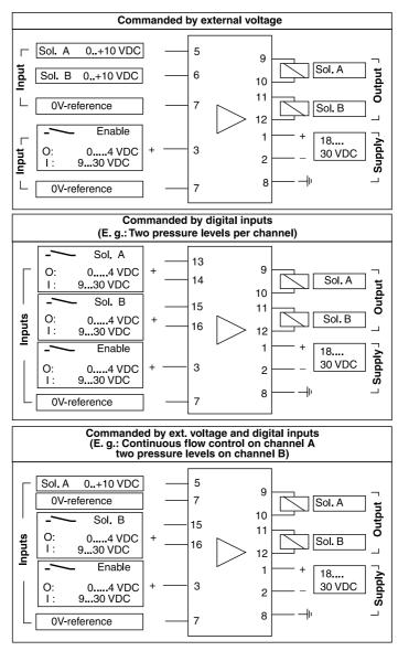
Certainly combinations and / or modifications of these examples are possible. The priority of the digital inputs over the analogue inputs has to be kept in mind! Via parameter N=1 all four digital inputs may be dedicated to channel A.
